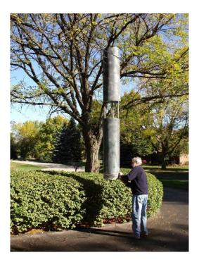
Dick, AH6EZ, adjusts the 160 Meter EH Missile—uh, antenna prior to the start of the Illinois QSO Party. Dick and Greg, N9CHA, both made 160 meter contacts with this low profile, stealth antenna.
