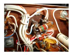
Bottom view of the old filter cap and resistors
