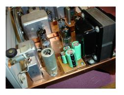
A right side view of the new filter capacitor.
