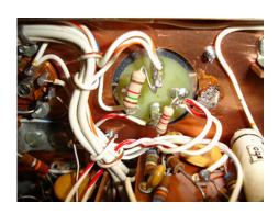
Bottom view of the new cap and resistors.
